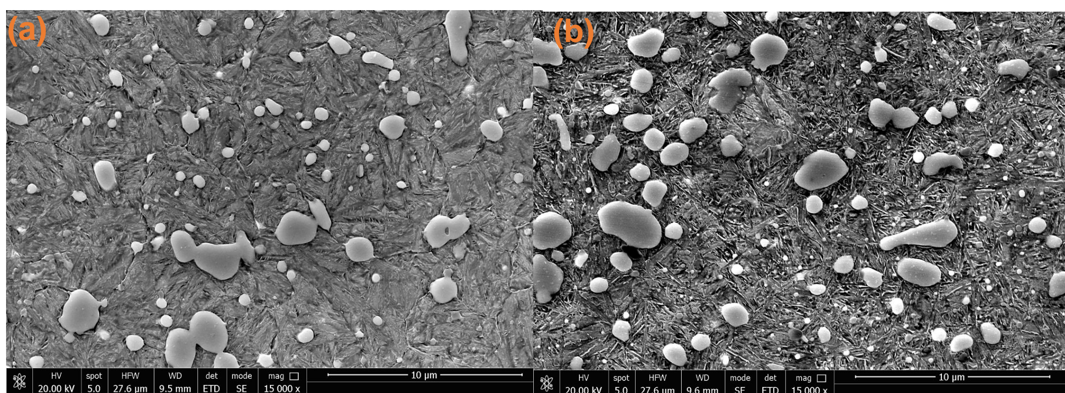
Fig. 2.1 – Scanning electron micrographs of the Microstructure of AISI M2 HSS in (a) as-quenched Q, and in (b) quenched & tempered followed by DCT, Q+T+DCT. Both consist of carbides in a martensite matrix
